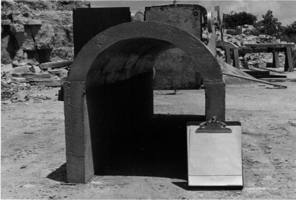
Figure 22. Type A tunnel constructed for Test Two, Phase One.
